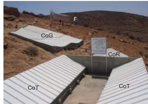
Figure 2: General view. CoT: condenser on terrace, 40.64 m 2 ; CoR: condenser on roof, 21.2 m 2 ; CoG: condenser on ground, 73.8 m 2 ; F: 40 m 2 fog collector.
