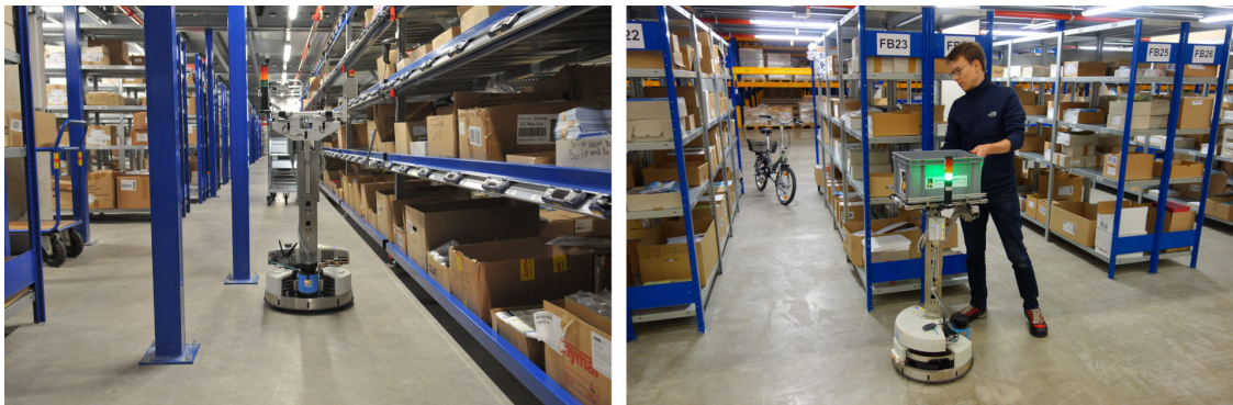
Figure 8.2.: Collaborative order-picking application in a warehouse environment. A fleet of robots assist human workers performing order-picking tasks.
