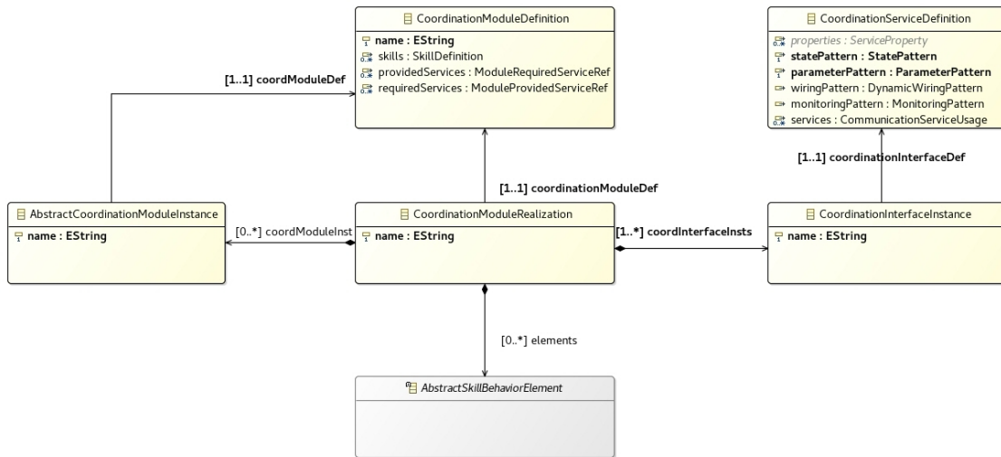
Figure 5.9.: Coordination module realization meta-model, binding the realization-independent module definitions to specific coordination interface instances.
