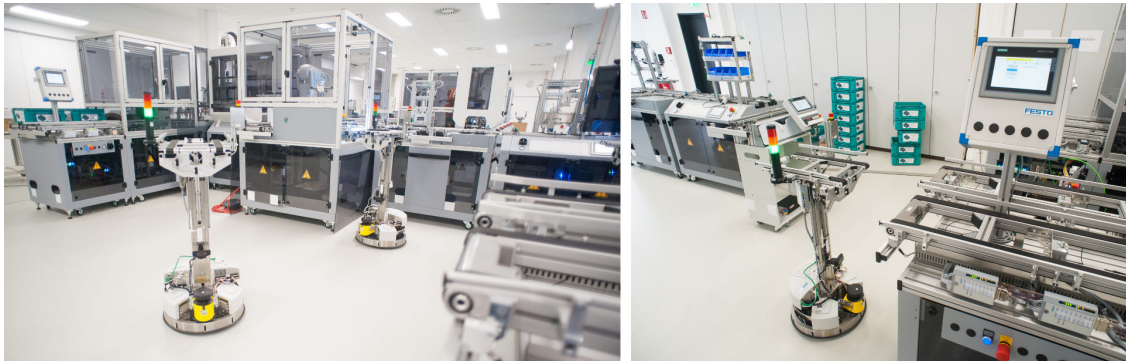
Figure 8.1.: Fleet of robots providing a transportation service between modular production stations.
