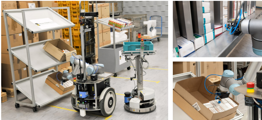
Figure 8.3.: Autonomous order-picking application in a warehouse. A fleet of heterogeneous robots perform order-picking tasks. A combination of manipulation robots (service robot Larry) and cheaper transportation robots (Robotino) is used to enhance the performance of the robot fleet.
