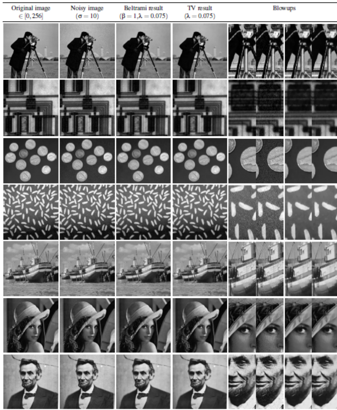
Figure 4.3: Beltrami and TV denoising applied to a larger set of test images. Asterisk denotes images shown in figure 4.3. Signal-to-noise ratio and structural similarity Index are in favor of the Beltrami model (bold). Also, the Beltrami model converges in a little more than half the iterations required for the TV model. Each iteration is only slightly more computationally complex than the TV algorithm, since both implementations are based on a very similar primal-dual projected gradient method and thus structurally identical. Convergence criterion is based on the decrease of the primal problem energy.
