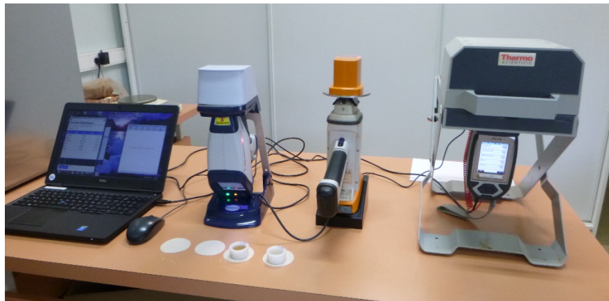
Figure 4. Presentation of the three pXRF devices and their stands during the measurement phase of wetted samples in the lab.
