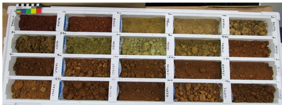
Figure 3. Drill chips from OUACO deposit prepared in a core tray divided into 20 cm compartments.
