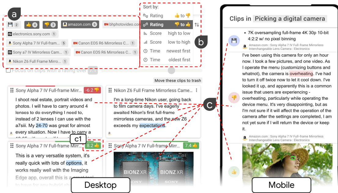
Figure 5.5: WiggLite’s information holding tank shown both on desktop and on mobile, which houses content that users collected through wiggling in the form of information cards (c). In addition, on desktop, users can apply different filters (a) and sorting mechanisms (b) to the information cards.
