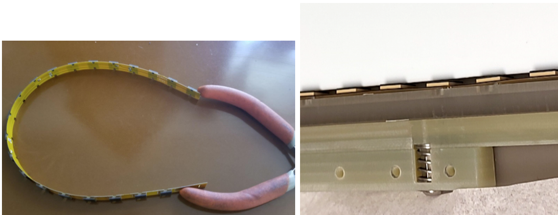
Figure 6.10: 20 SiPMs mounted to flexible PCB (left). Flexible PCB positioned against a dummy WLS plate (white block) with spring-loaded dynamic mount (right).
