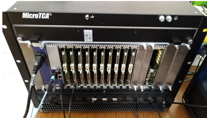
Figure 4.20: \mu TCA crate with a 40 Gbit/s MCH.
