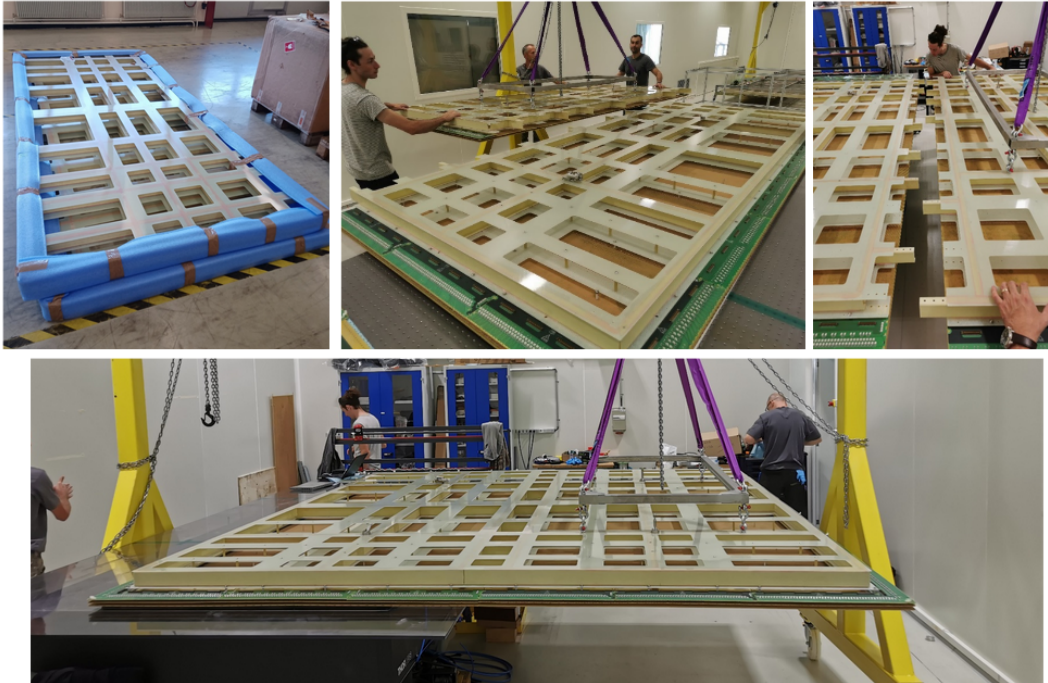
Figure 3.37: Top Left: Two halves of the composite frame as received from the manufacturer. Top Middle: Half composites are attached to the anode assembly and they are ready to be connected. Top Right: Connecting two half units. Bottom: Composite frames are connected and assembly is ready for the edge card installation.
