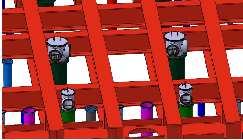
Figure 4.38: 3D view of the cryostat roof I-beam structure and the position of both the larger and smaller chimneys.
