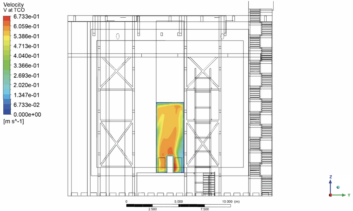
Figure 9.15: CFD model of the air flowing out through the TCO with 16,000 CFM of pure filtered air entering through the West access hatches in the cryostat roof. The velocity is consistently above v_{air} > 0.2 m/s.
