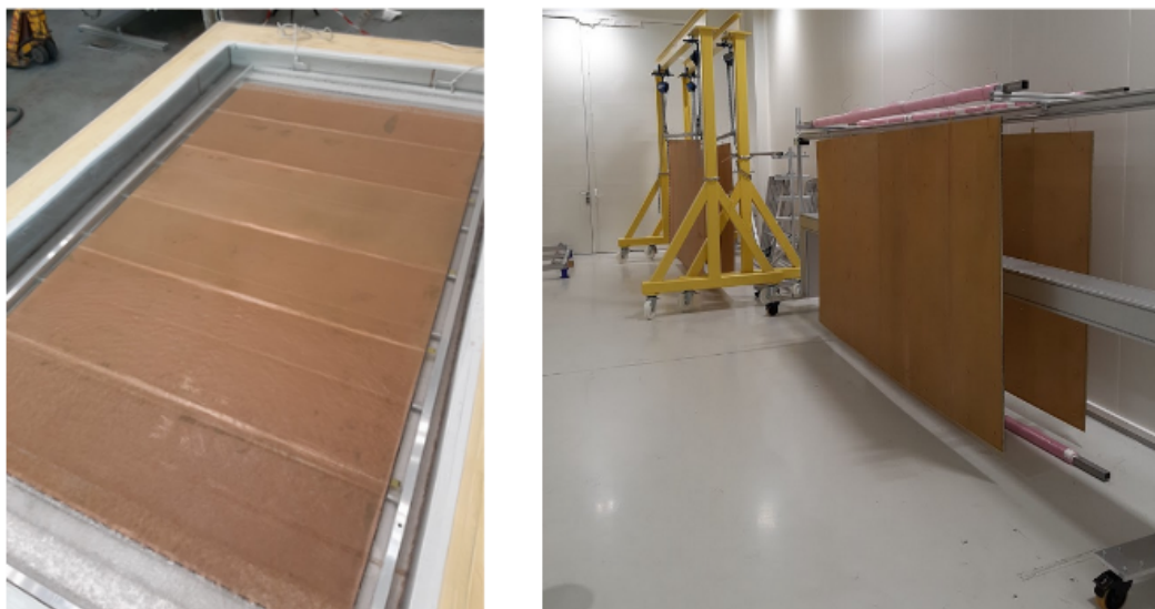
Figure 3.36: Left: Cryogenic test of the glued and silver printed PCB panel. Right: Drying in the clean room after final cleaning prior to assembly.
