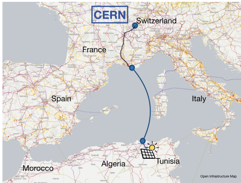
Figure 3.4: Potential CERN-LINK cable (in blue) connecting North African solar power plants with the European electricity grid. Also shown are existing power lines (purple, red, dashed blue), gas and oil pipelines (green/yellow) and PV plants (yellow/red dots). Base map taken from Ref. [104], reused and annotated under the terms of the Creative Commons Attribution 4.0 International (CC BY 4.0) license .
