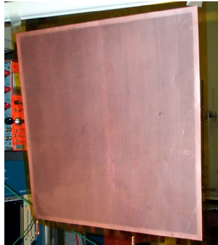
Figure 2.28: Left: GEM DHCAL Concept. Right: A 30 cm x 30 cm foil from 3M Corporation.
