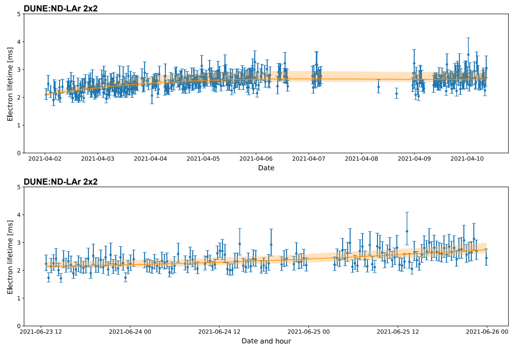
Figure 28. Extracted electron lifetime as a function of time during Module-0 Run 1 (top) and Run 2 (bottom), with the average uniformly exceeding 2 ms in both cases.
