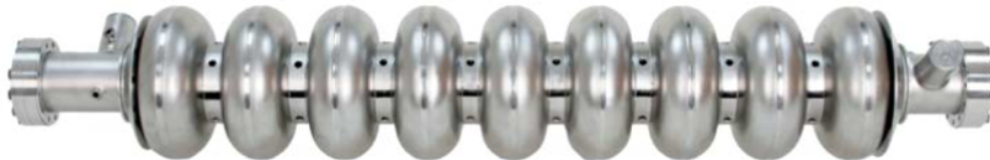
Figure 4.1. TESLA 1.3 GHz nine-cell SRF cavity
