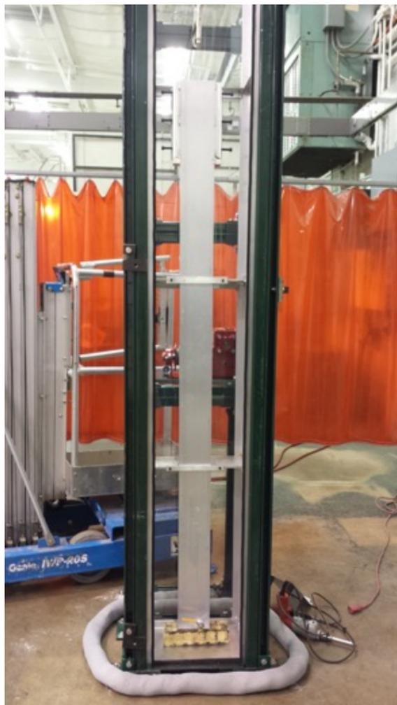
**Figure 40:** Mechanized dipping setup at Fermilab, used for the production of dip-coated light guides.
