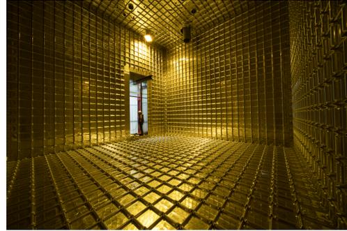
**Figure 4:** Left: the GTT inner vessel layers. Right: view of the inside of the cryostat ProtoDUNE-SP just after the finalisation of the primary membrane installation. The gold hue visible in the picture is an artifact of the lighting used during the installation, to protect the PDS.
