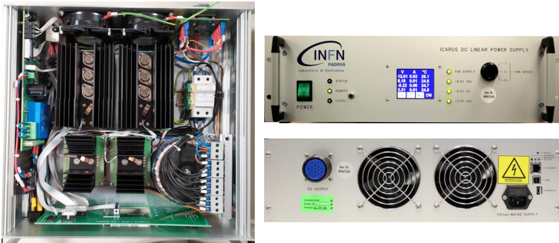
Figure 4. Inside (left) and front and rear panels (right) of the ICARUS LVPS module.
