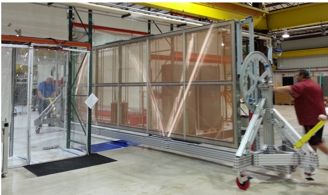
Figure 2.35: A ProtoDUNE-SP APA being moved around the PSL production facility on a process cart.
