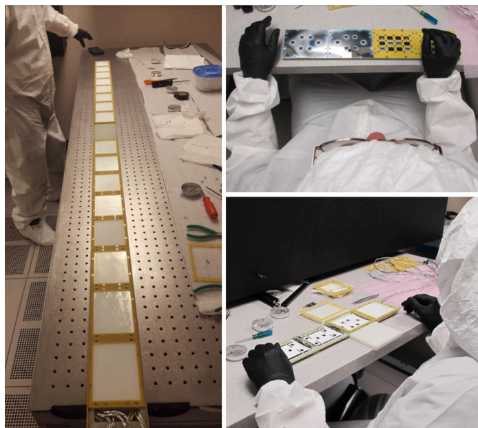
Figure 5.23: ProtoDUNE-SP S-ARAPUCA module being assembled in a class 100,000 clean area. Front face of assembled module (left) shows the 16 coated dichroic filter plates. Assembly photos show the reflective rear side (top right) and inner coated surface (right bottom) of Vikuiti reflective foils. Note the cutouts in foil for MPPC active area.
