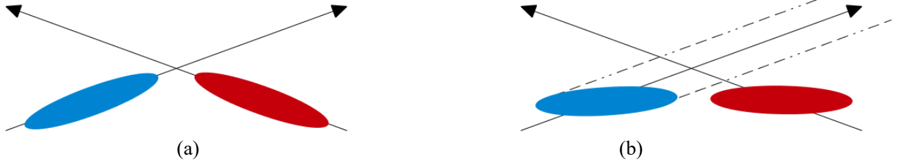
Figure 4-1: Bunches colliding with (a) a crossing angle without crab crossing; (b) with the crab crossing
