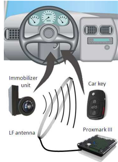
Figure 7.4: Experimental setup for eavesdropping
