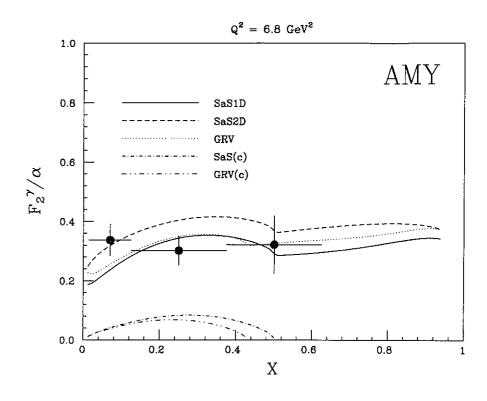
Figure 2: The  $F_2^{\gamma}$  values as a function of x. The data (closed circles) are compared with the SaS1D(solid), SaS2D (dashed) and GRV (dotted) model predictions. The heavy quark contributions for the SaS (dot-dashed) and the GRV (double-dot-dashed) models are shown separately.
