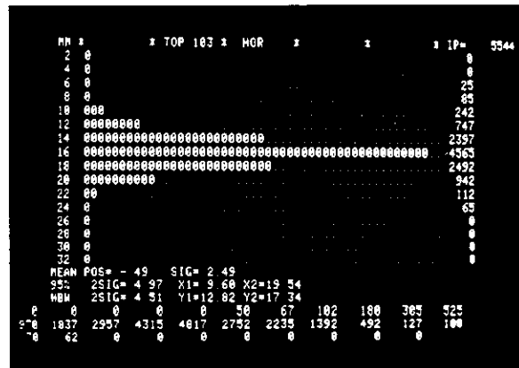
Fig. 17 Horizontal beam profile from toposcope 103 (during 2.1 \mu s, corresponding to 1 ejected turn)
