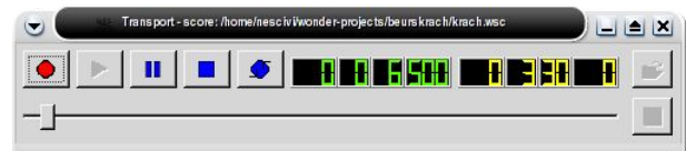
Figure 3. Transport control of WONDER. The slider enables the user to jump to a new time. The time in green (left) indicates the running time, the time in yellow (right) the total duration of the score. The caption of the window indicates the name of the score file.
