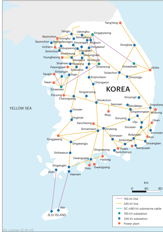
Figure 1: Electric infrastructure in Korea
