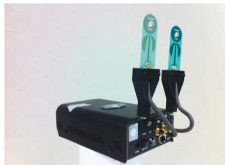
Figure 1 Time Domain UWB P220 in Monostatic mode.
