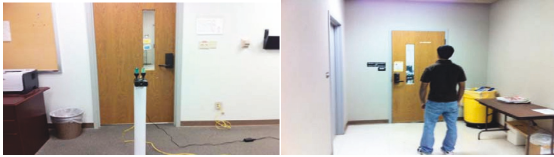
Figure 3 UWB radar (Left), Human target (Right) for wooden door.
