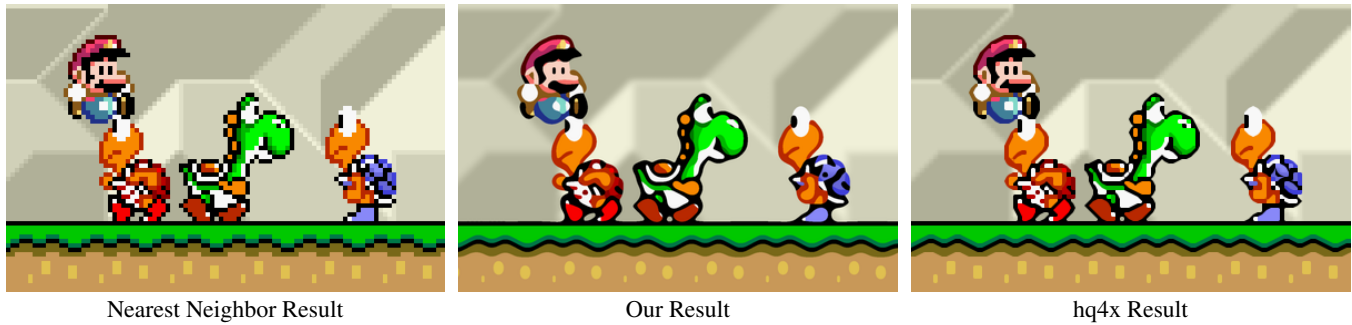
Figure 10: Applying pixel art upscaling in a dynamic setting. The output frame of an emulator is magnified by 4\times (crop shown). Please zoom into the PDF to see details (Image © Nintendo Co., Ltd.).
