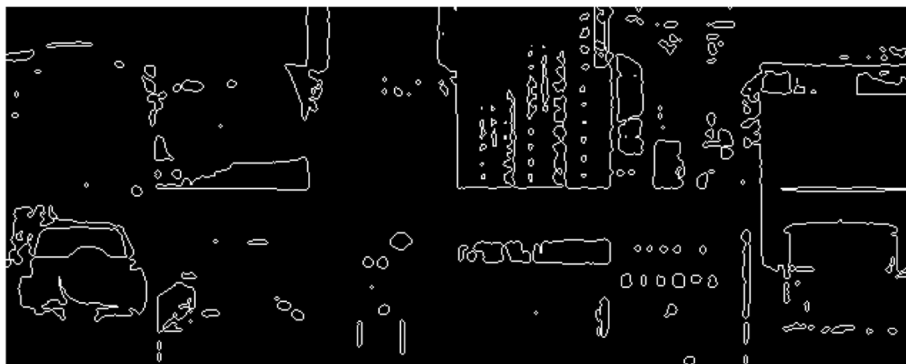
Fig. 12 Results of edge detection of obstacles ahead combined the gray average with the Laplacian operator
