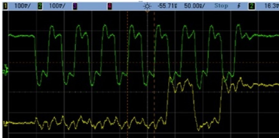
Fig. 37 The interrupt waveform of gyro sensors INT
