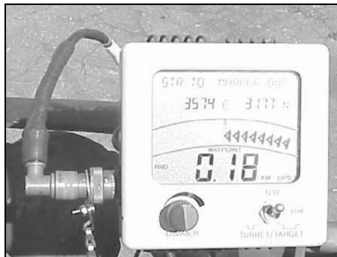
Figure 6-18. Driver's display showing steering directions, distance, and position
