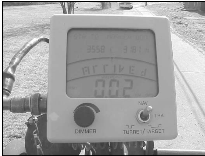
Figure 6-19. Driver's display showing arrival at the waypoint
