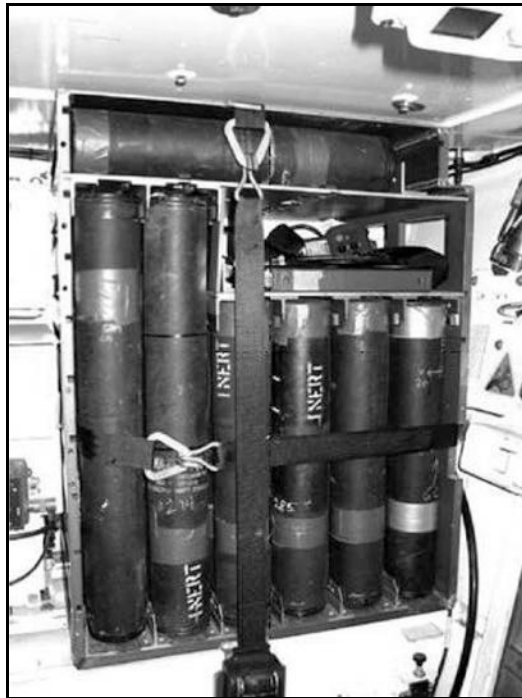
Figure 5-29. Right side ammunition rack
