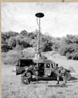
OCT. The Army deployed a prototype of the Prophet system to support Operation ENDURING FREEDOM. The Prophet is the Army's next generation, multi-discipline collection, jamming, processing, and reporting system.
