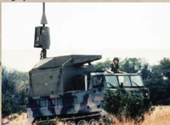
Army units in Korea and Europe field the TEAMPACK (AN/MSQ-103A), a ground direction-finding system.
