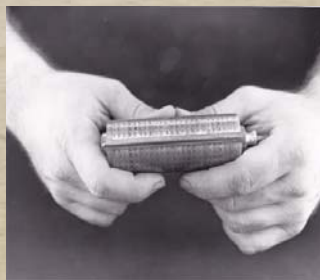
The Army adopted the M-94 Cylindrical Cipher Device, providing field units with a practical communication security device.
