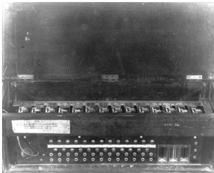
The SIS used this analog of the Japanese Purple machine to decipher Japanese diplomatic messages in 1940.
