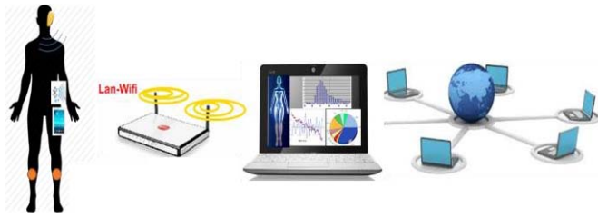
Fig. 3. Sketch of System 2: the two sensors are positioned on the shins, a smartphone is used as portable receiver, a headphone is wireless connected for the auditory feedback, a PC is connected to the smartphone via the wifi. The information and database can be shared in a cloud.
