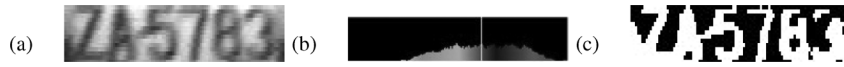
Fig. 15. Invident difference between the colors of the characters and the background. (a) Compact plate region. (b) Histogram. (c) Binary representation after thresholding by Otsu's method.
