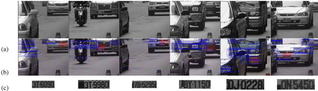
Fig. 22. Examples of a variety of plates on a cloudy day. (a) Input images. (b) Recognized results shown in color images. (c) Enlarged recognized plates.
