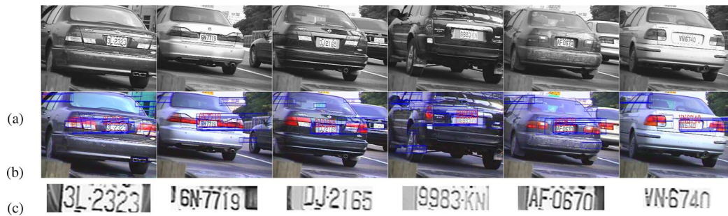
Fig. 25. Examples of a variety of plates captured from a device installed in a car. (a) Input images. (b) Recognized results shown in color images. (c) Enlarged recognized plates.
