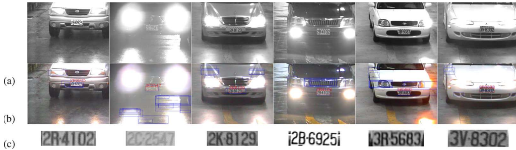
Fig. 21. Examples of a variety of plates on a wet day. (a) Input images., (b) Recognized results shown in color images. (c) Enlarged recognized plates.
