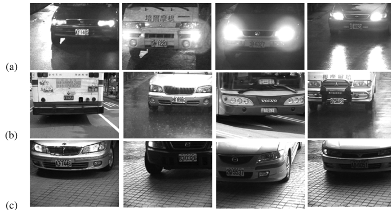
Fig. 2. Examples of variations in plate types and environments. (a) Different vehicle headlights. (b) Different types of environment lighting. (c) Plate-like background.
