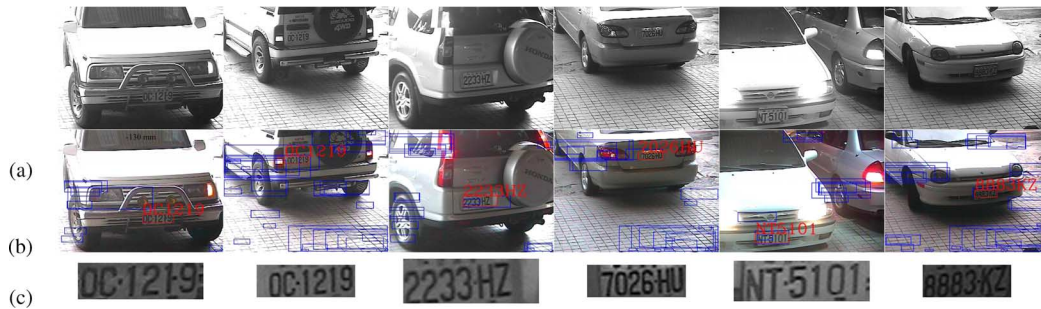
Fig. 24. Examples of a variety of plates with the pavement background of texture patterns. (a) Input images. (b) Recognized results shown in color images. and (c) Enlarged recognized plates.
