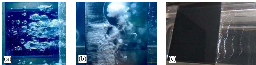
Fig. 1. Types of cavitation on a 2D hydrofoil (flow from left to right): (a) travelling bubbles, (b) unstable attached sheet and (c) Von Karman vortex-shedding.
