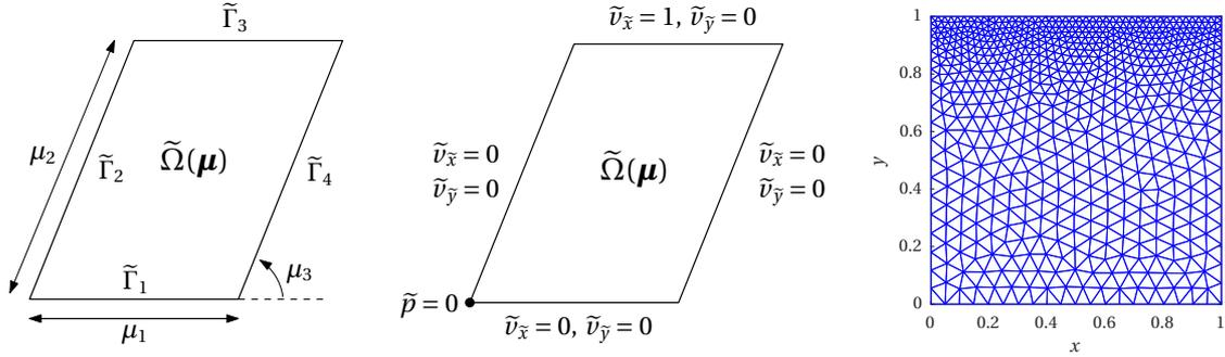
**Figure 6.8.** Computational domain  $\tilde{\Omega}(\boldsymbol{\mu})$  (left), enforced velocity at the boundaries (center) and computational mesh  $\Omega_h$  (right) for the lid-driven cavity problem for the incompressible Navier-Stokes equations.
