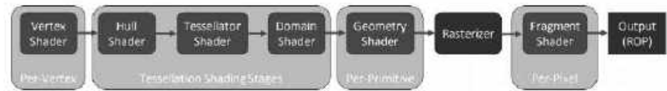
Figure 2.2: Rendering pipeline in depth. The gray boxes are programmable shaders and the black boxes are fixed stages. Adapted from (Wyman and Marrs 2019).
