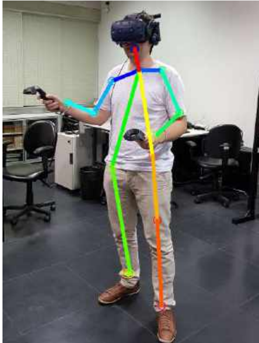
Figure 4.7: Pose Detection and Motion Capture: currently Head and Hands are captured using HTC Vive Headset and Controllers; in future implementations the user's pose (indicated by the superimposed skeleton) will be estimated and tracked by the AI method described in (L. J. S. Silva et al. 2019).
