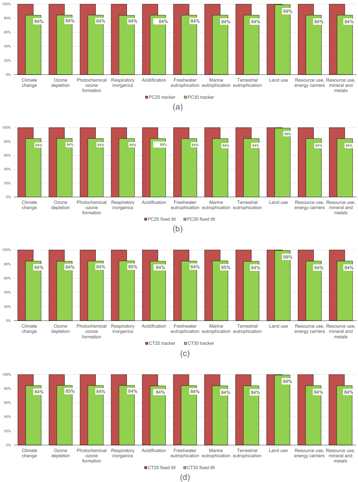
Figure 8: LCIA of ground mounted PV electricity with PERC modules (FU 1kWh). Lifetime sensitivity analysis: (a) PV plant located in Piacenza with tracker; (b) PV plant located in Piacenza with modules at fixed tilt; (c) PV located in Catania with tracker; (d) PV plant located in Catania with modules at fixed tilt. Impacts for the 30-year scenario are expressed as a percentage of impacts for the 25-year lifetime scenario.
