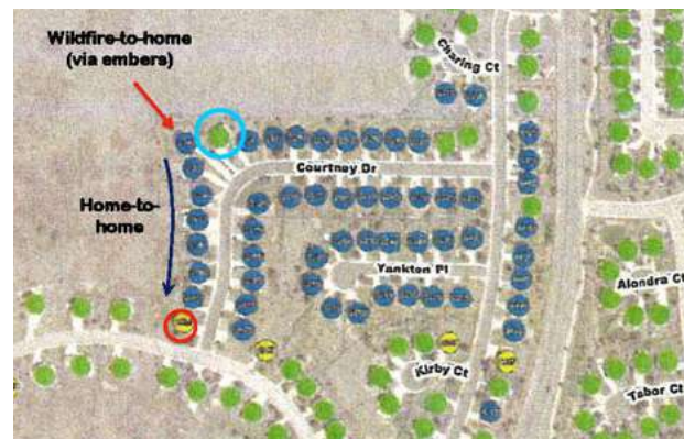
Figure 14: Homes on Courtney Drive that were destroyed by home-to-home spread after an initial wildfire-to-home ignition (indicated with red arrow). One home at the top of slope (red circled) suffered minor damage. The home to the east (right) of the wildfire-to-home, shown as a non-damaged green dot in this figure (blue circled), also had minor damage. Source: IBHS.
