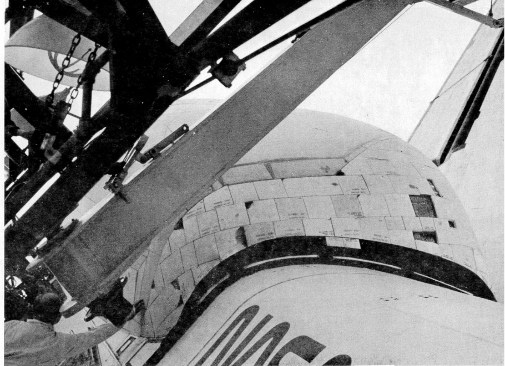
Figure 2-27.- Scorching of tile on forward edge of OMS pod.
