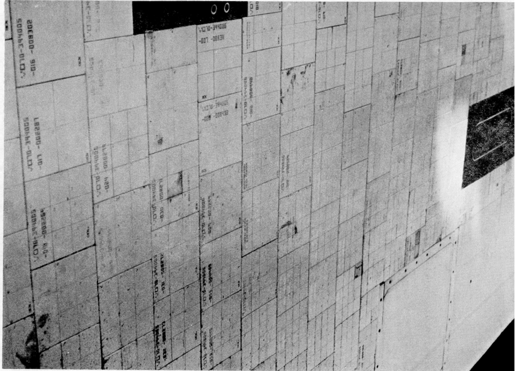
Figure 2-24.- Coating loss caused by unknown contaminant.
