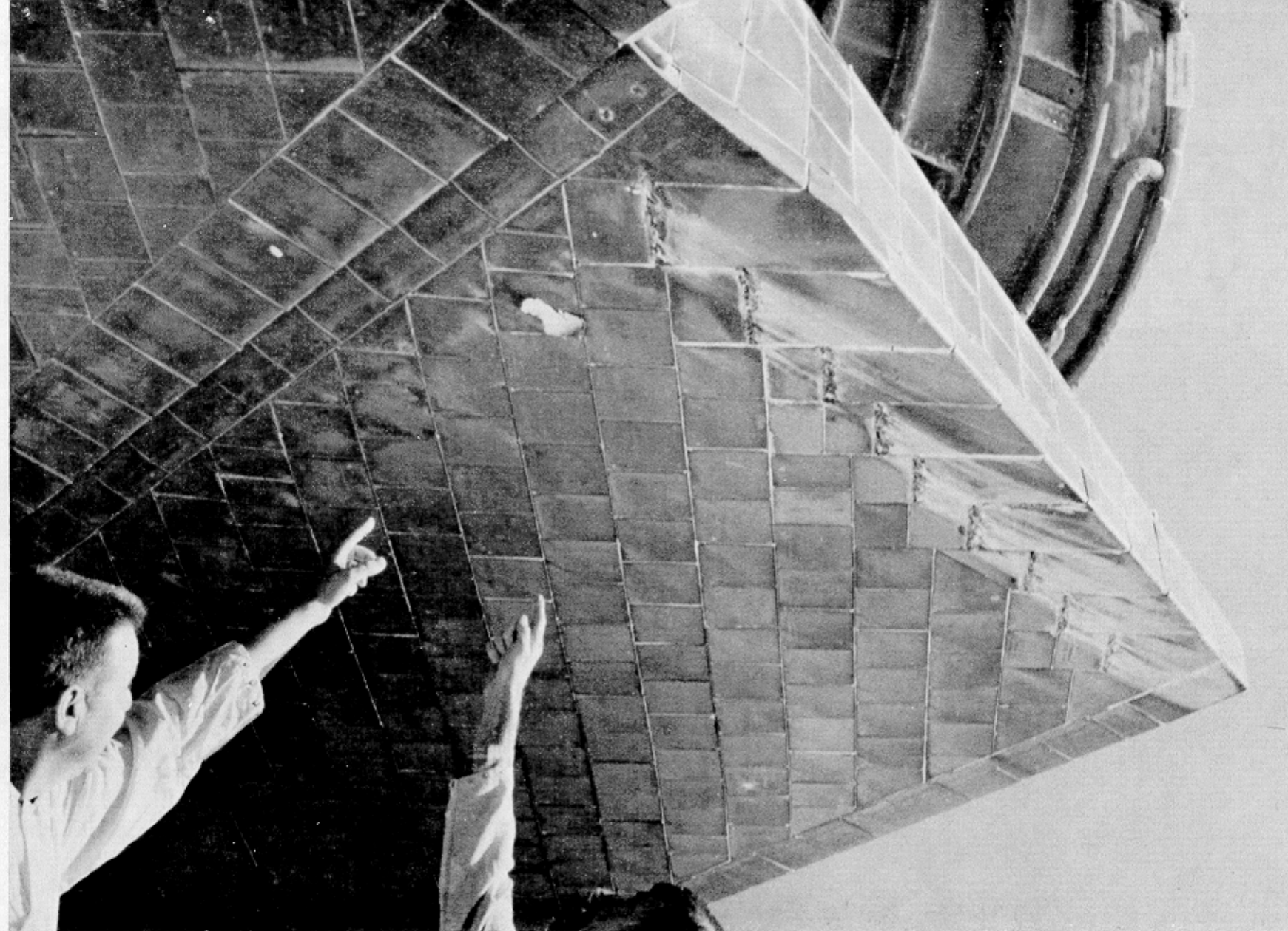
Figure 2-23.- Impact damage to left lower forward region of body flap.
