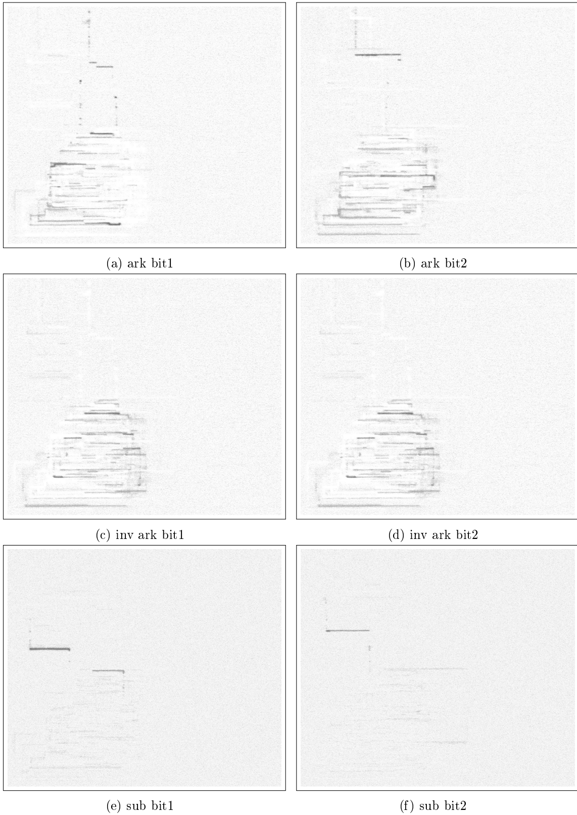
Figure 3.7: Different correlation images found in clock cycle 42; addroundkey, inverted addroundkey and subbytes. The colors are inverted for improved visualisation.
