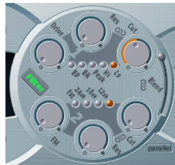
Parallel filter signal flow
