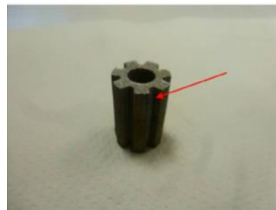
Figure 4. Fabrication of the primary wick, (a) printing procedure highlighting the laser points; (b) final result with a scaffold porosity of 17% [38].
