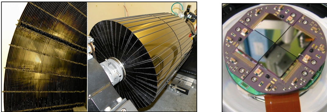
Figure 2 Left - Photographs of one of the two optics modules. Each mirror assembly has 133 shells. Right - One of the two detector modules with 4 CZT detector crystals. Each detector crystal measures 2cm x 2cm and contains an array of 32x32 independently discriminated pixels.
