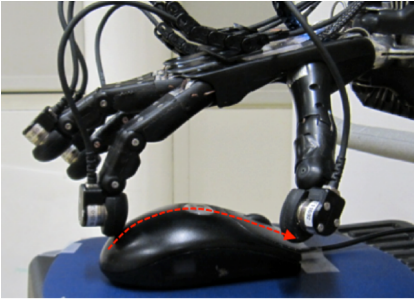
Figure 26: Surface contour following using the contact sensing finger (control diagram). [160]. Range_{des}(|f_d|_r) is a range of the desired force, (|f_n|_m) is the measured normal force, (|f_n|_r) is the friction cone, (f_n) and (f_t) are the normal and tangential forces, P is the contact point location, and (J^{-1}) is the robot's inverse kinematics.
