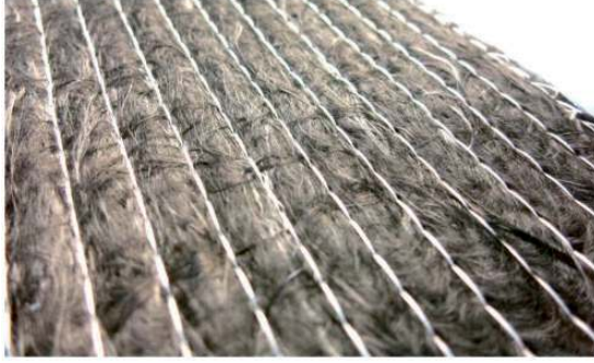
Figure 1. Reclaimed carbon fibre dry material used in this study. Short randomly poorly oriented fibres are stitched together to form a mat.
