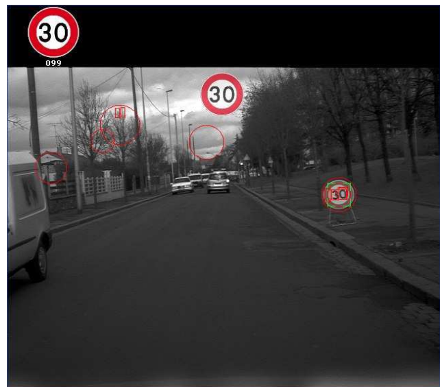
Fig. 9. Example of speed-limit sign detection on a E.U. street. All detected circles are shown (in red), and the candidate digits segmented inside them are outlined in red. The speed signs recognized on the current image are shown on the top black zone, with their associated confidence, and the currently validated speed limit is superimposed on top-center of image.
