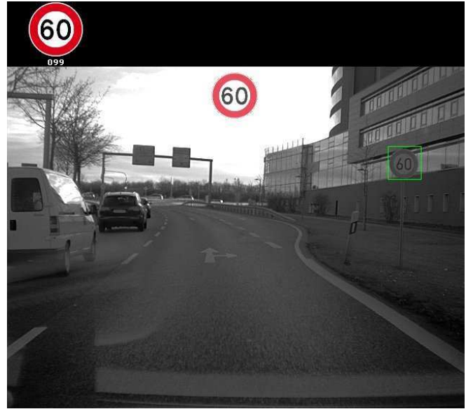
Fig. 11. Correct recognition of a German speed-limit sign illustrating promising results for pan-European speed-limit recognition.
