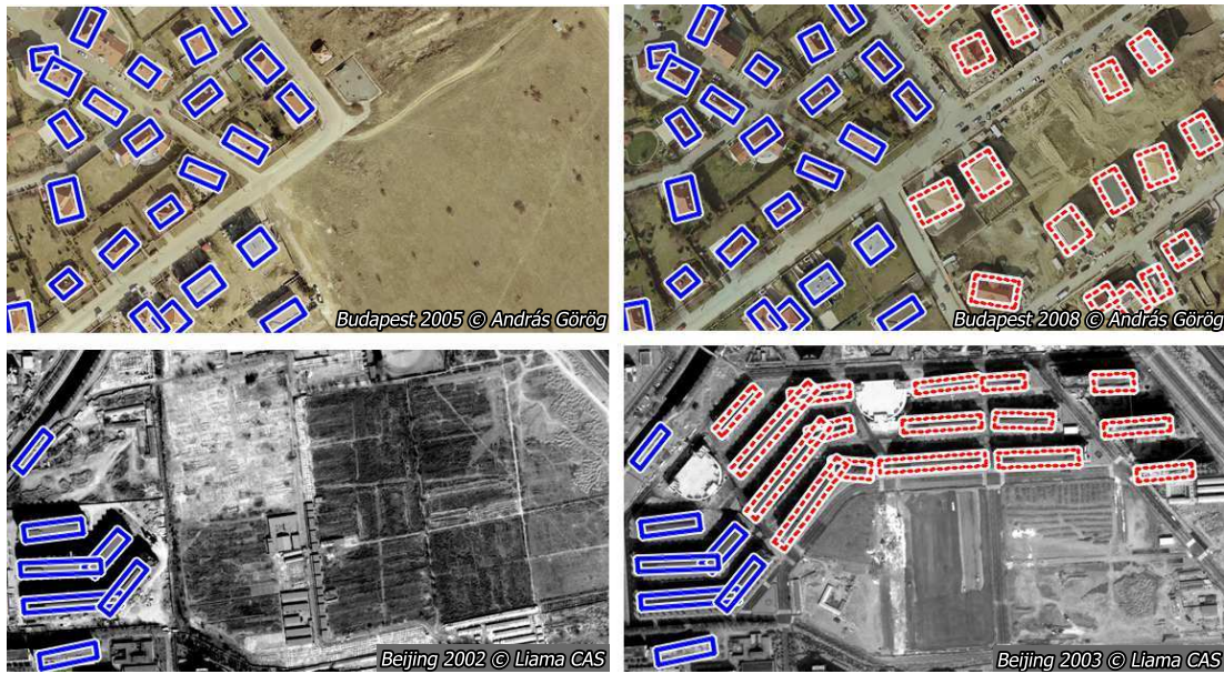
Fig. 26. Results on BUDAPEST (top, image part - provider: András Görög) and BEIJING (bottom, provider: Liama Laboratory CAS, China) image pairs, marking the unchanged (solid rectangles) and changed (dashed) objects
