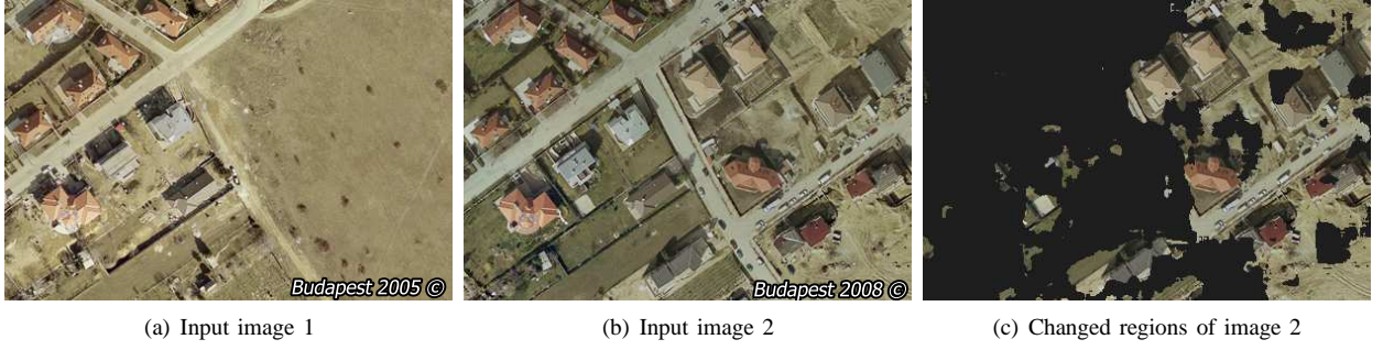
Fig. 6. Low level change detection: (a) and (b) input images, (c) Bhattacharyya change mask q_{ch}
