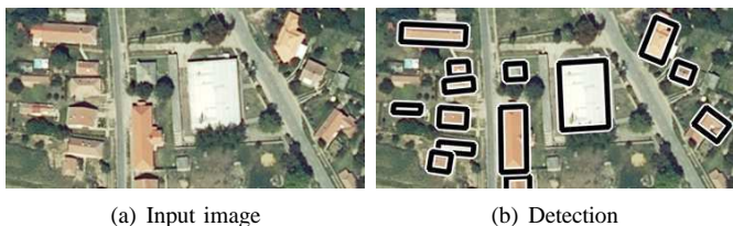
Fig. 17. Detection results in case of significantly different building scales, using the features from Fig. 16
