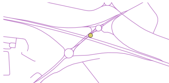
Figure 5. Two representations of highway interchanges (road lines and points) in a MRDB, that can be used to generate a training dataset to classify images that contain highway interchanges.
