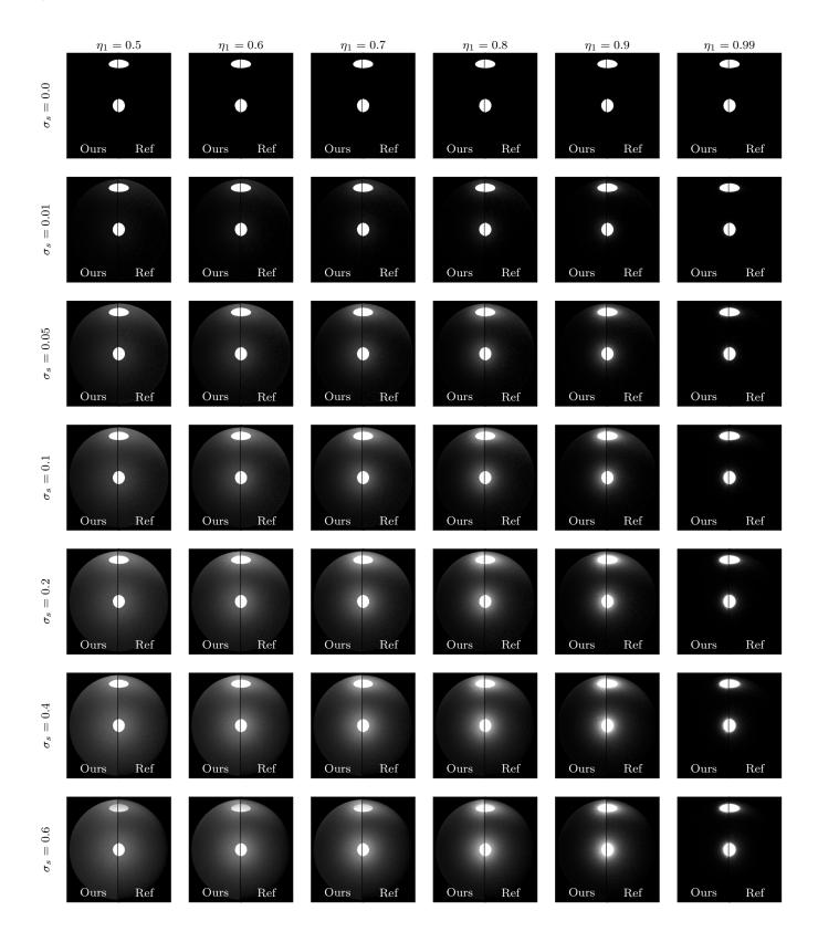
We also validated the ability of our method to match the reference when rendering participating media of increasing optical depth (using  $h \in [0,0.4]$ ) with an environment map lighting. In this scene, we use a pure mirror as the base layer on top of which a medium of increasing depth is applied. We specified  $\sigma_a = 0$ ,  $\sigma_s = 1$  and, g = 0.9 as constants for the medium. As shown below, our method faithfully reproduce the stochastic reference in such context.
