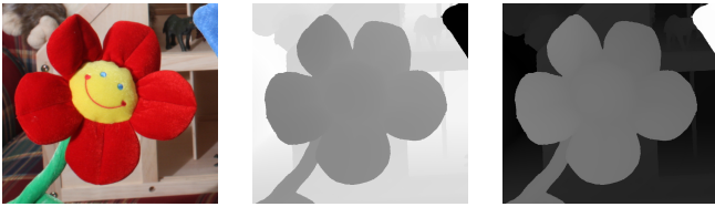
Fig. 2. Example of a color image (excerpt from the Flowers image), its corresponding depth-map (middle) and its corresponding disparity-map (right).
