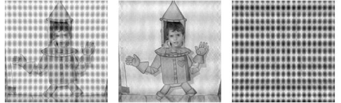
Fig. 4. Left: Original signal. Middle: First morphological component (curvelet transform) extracted with MCA/MOM. Right: Second morphological component (global DCT) extracted with MCA/MOM.
