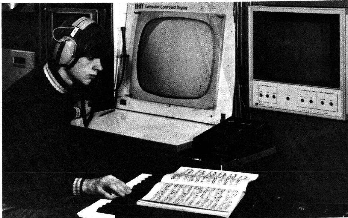
Fig. 2 Music can be Entered Directly into the Computer Memory from an Organ Keyboard
