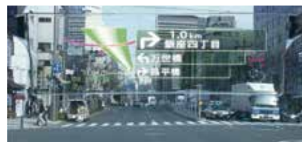
Pioneer’s HUD projects augmented-reality (AR) information beyond the windshield through laser scanning using MEMS mirror.
