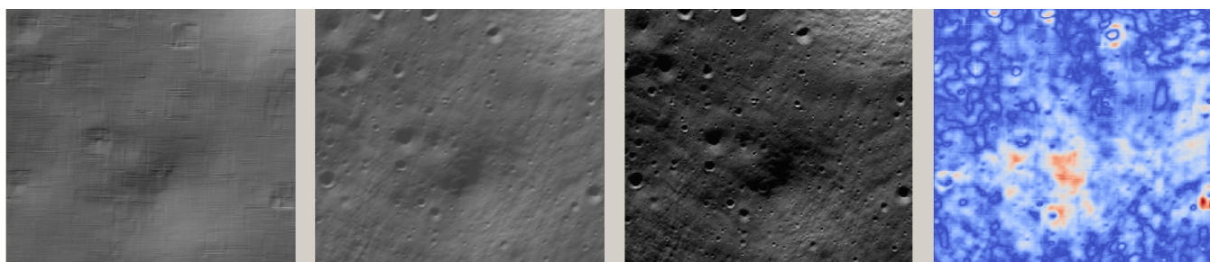
Figure 10.1: An illustration of sfs . The images are, from left to right, the original hill-shaded DEM, the hill-shaded DEM obtained from sfs , the image A.cub map-projected onto the original DEM, and the absolute difference of the original and final DEM, where the brightest shade of red corresponds to a 2 meter height difference.
