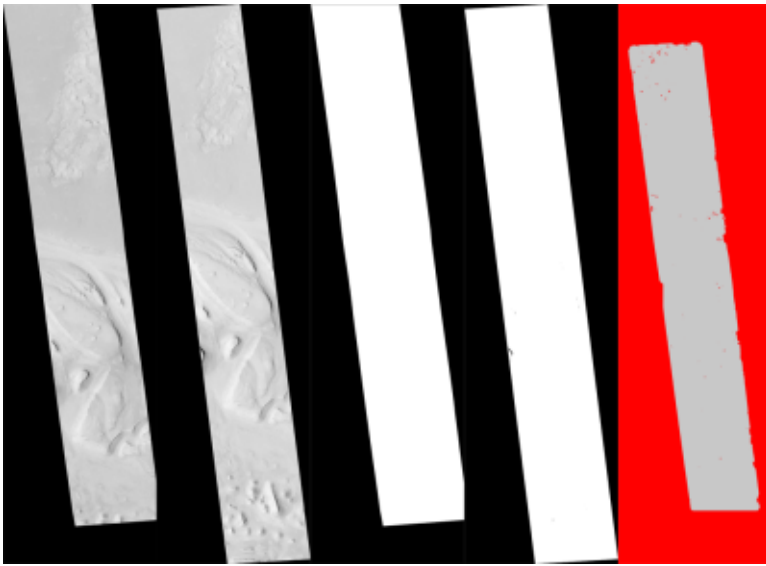
Figure 5.1: These are the four viewable .tif files created by the stereo program. On the left are the two aligned, pre-processed images: ( results/output-L.tif and results/output-R.tif ). The next two are mask images ( results/output-lMask.tif and results/output-rMask.tif ), which indicate which pixels in the aligned images are good to use in stereo correlation. The image on the right is the “Good Pixel map”, ( results/output-GoodPixelMap.tif ), which indicates (in gray) which were successfully matched with the correlator, and (in red) those that were not matched.
