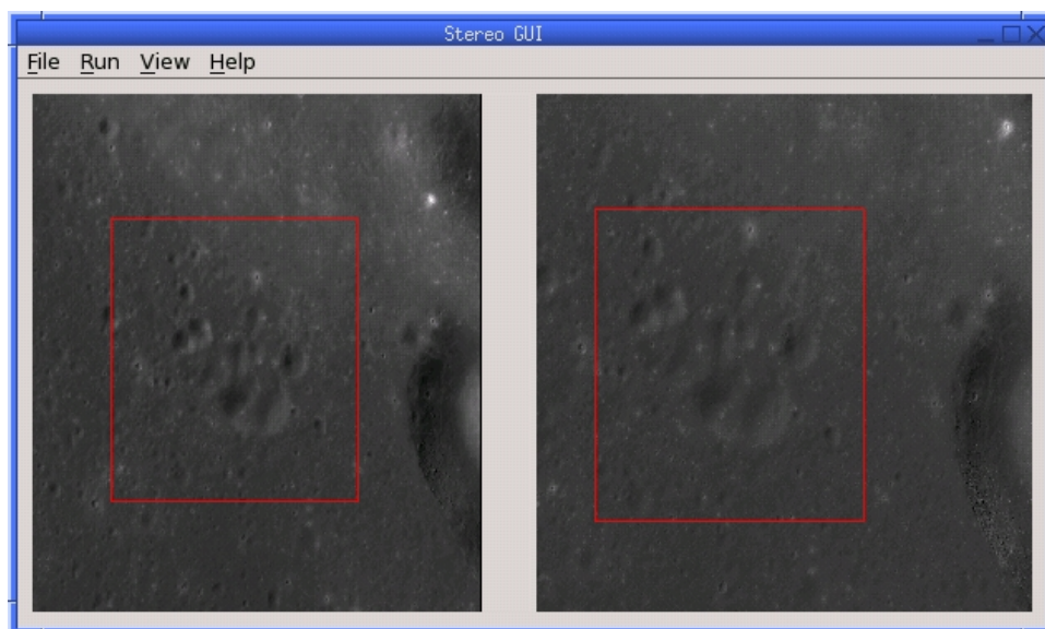
Figure A.1: An illustration of stereo_gui . The stereo command will be run on the regions selected by red rectangles.
