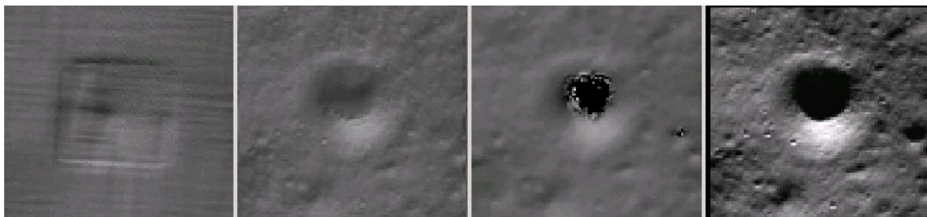
Figure 10.2: An illustration of sfs . The images are, from left to right, the hill-shaded initial guess DEM for Sfs, the hill-shaded DEM obtained from sfs , the “ground truth” DEM, and the first of the images used in Sfs map-projected onto the optimized DEM.
