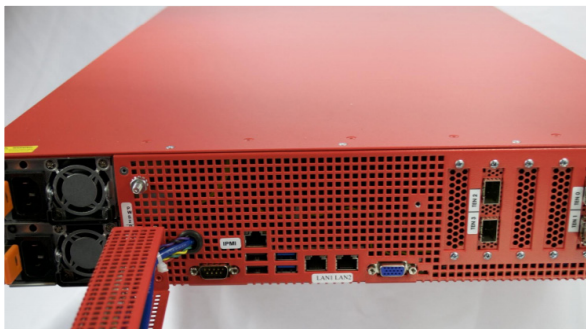
40Gb/s OCA Storage Appliance with 248TB storage (2RU form factor)
