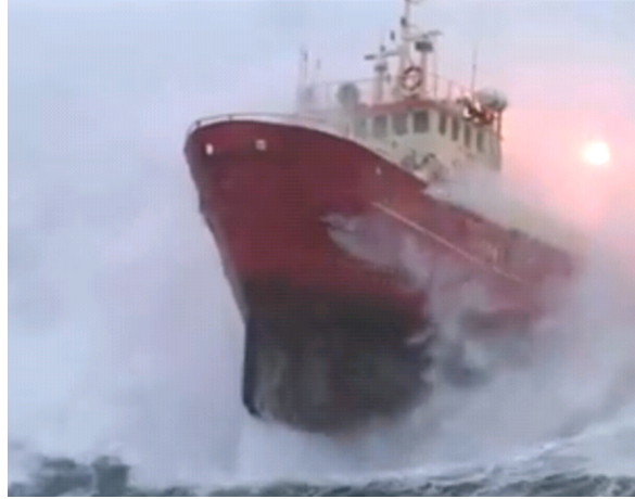
Figure 1: A ship in high sea. The wave forces can result in very high accelerations in the ship motion. (© 2010 IEEE)
