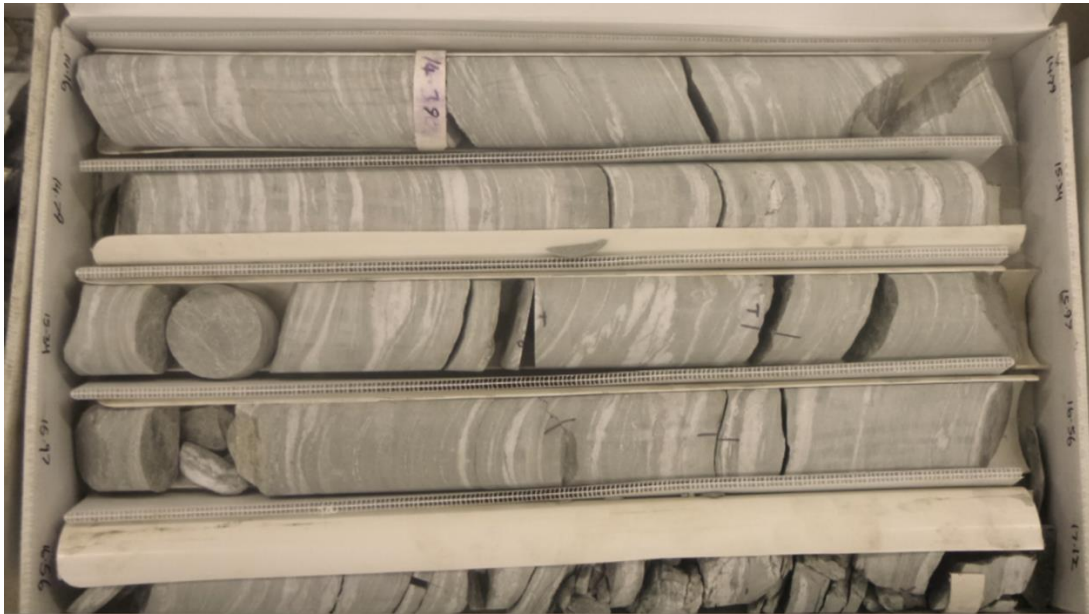
Figure 1: Photo of typical retrieved core specimen showing foliation patterns
