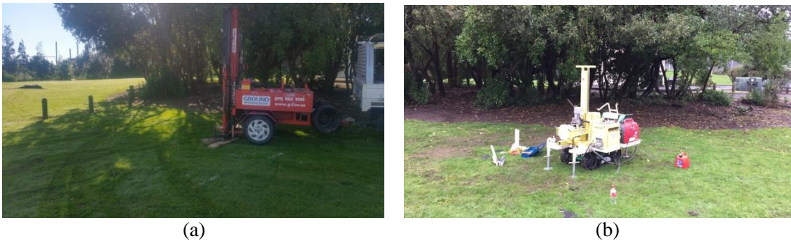
Figure 2: Field testing at Target site #1: (a) CPT and sCPT; and (b) SDS test.
