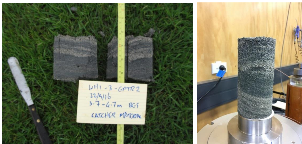
Figure 7: Samples of soils taken at site #1. White-coloured layers are pumiceous, while dark-coloured ones are hard-grained sands.
