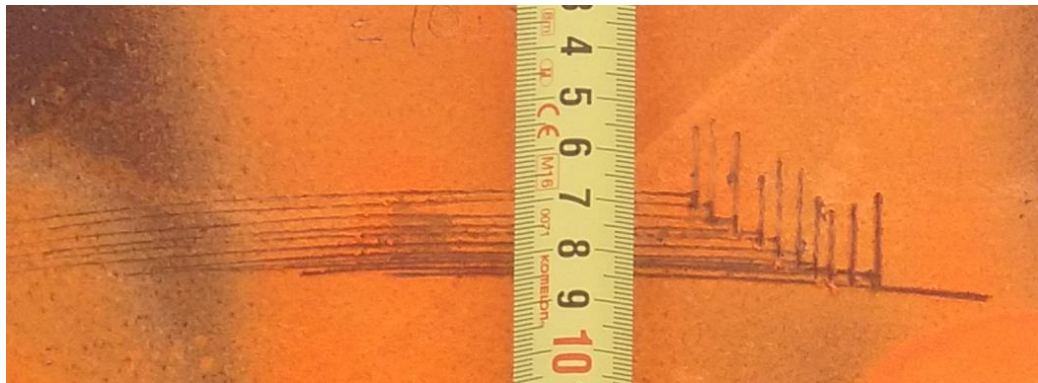
Figure 3: Example of manual set card on steel pile
