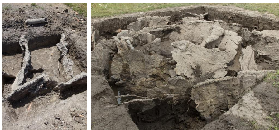
Figure 1. Hand-exhumed resin veins (left) and hydro-exhumed resin veins (right).
