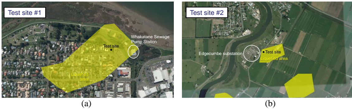
Figure 1: Target sites for the study: (a) Test site #1 near Whakatane Sewage Pump station; and (b) Test site #2 near Edgecumbe substation. Yellow hatched zones are the regions where liquefaction had been observed based on literature.
