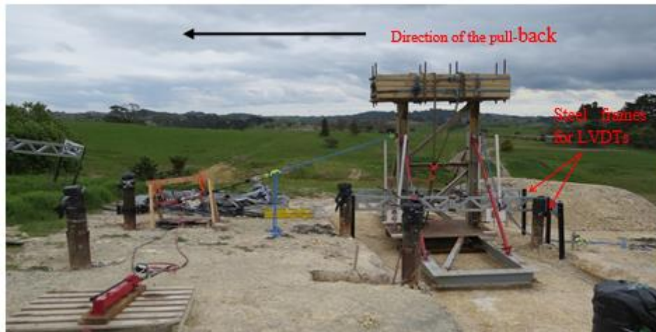
Figure 3: Experimental set-up assembled on site for snap-back test
