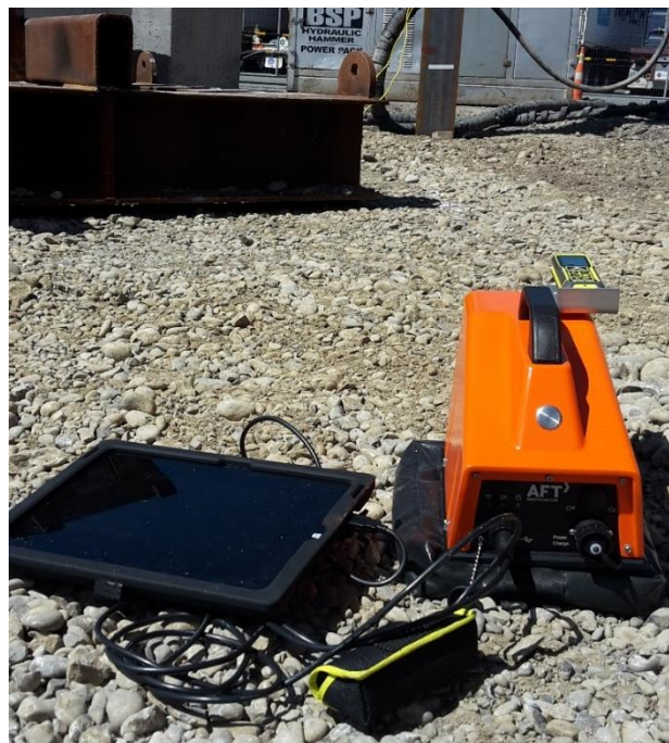
Figure 4: PDM set up outside exclusion zone
