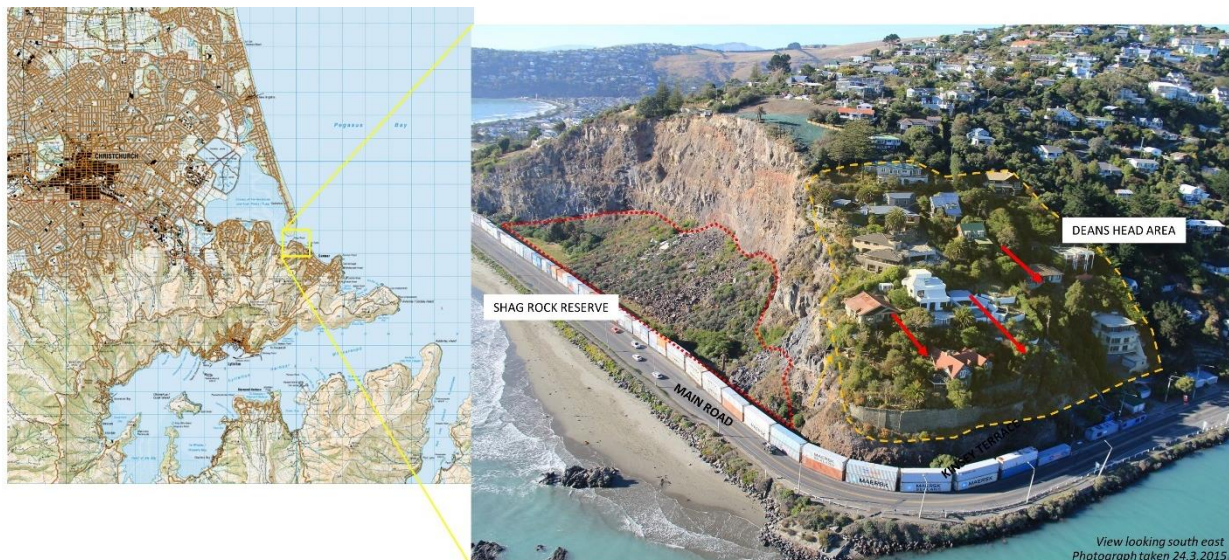
Figure 1: Deans Head and Shag Rock Reserve site areas in relation to Main Road. Indicative movement direction shown in red arrows (LINZ, 2011 and Aurecon, 2015).
