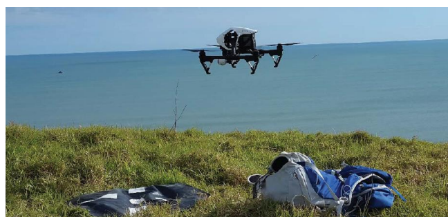
Figure 2: DJI Inspire 1 UAV taking off near a black and white GCP (Ohuka Landslide).
