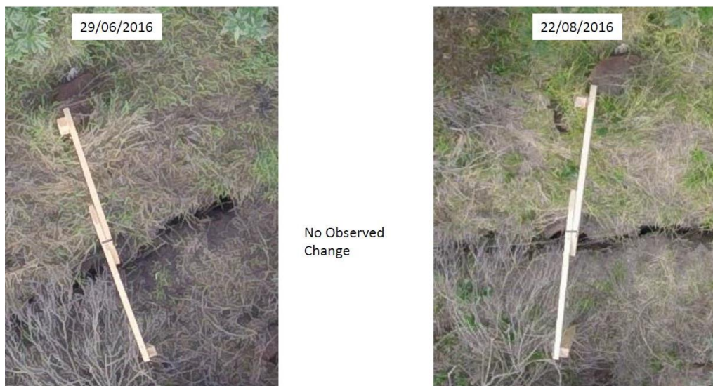
Figure 2: Comparison from UAV images of tell-tale monitoring at Shag Rock Reserve (Aurecon, 2016a).
