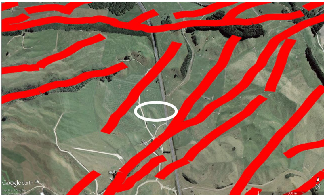
Figure 4: Active faults in the Tumunui area (New Zealand Active Faults Database, 2016). White ellipse indicates section of road affected by tomos.
